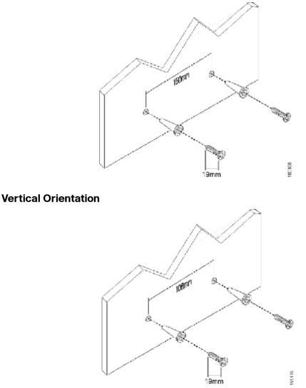
**STEP 2** Insert the screws, leaving a gap of 4mm between the screw head and the wall. Then mount the Cisco UC320W as shown.
