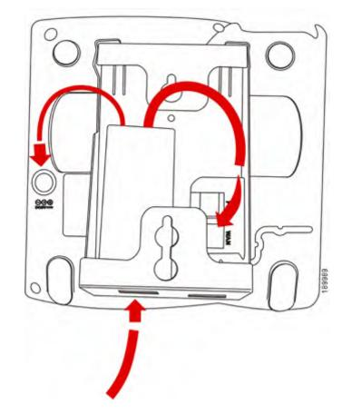
**STEP 5** Plug in the Ethernet and power cables.
