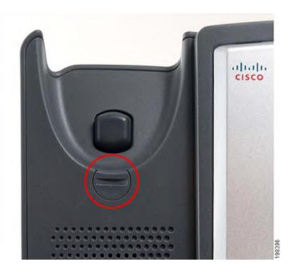
• **Cisco SPA500 Series models:** Push the latch in. Slide the retention tab up until it detaches from the phone. Rotate the tab 180 degrees and re-attach it.
