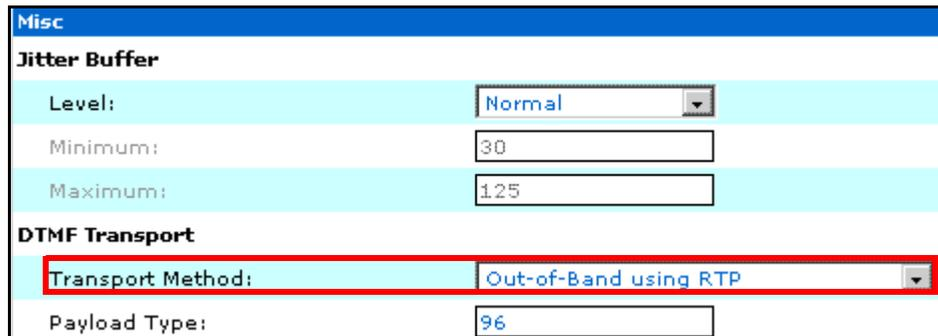
The screenshot shows the 'Misc' configuration page. Under the 'Jitter Buffer' section, the 'Level' is set to 'Normal', 'Minimum' is 30, and 'Maximum' is 125. Under the 'DTMF Transport' section, the 'Transport Method' is set to 'Out-of-Band using RTP' (highlighted with a red box), and the 'Payload Type' is 96.
